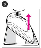
Turn unit to standby mode and unplug. When cooled, remove Ultra-Microfiber pad.
